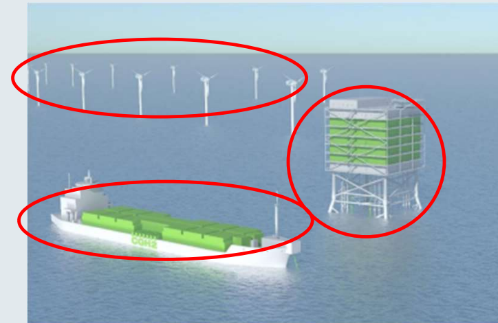
Schematic illustration of an offshore concept for hydrogen production and pressurised gas transport (ship or pipeline)
